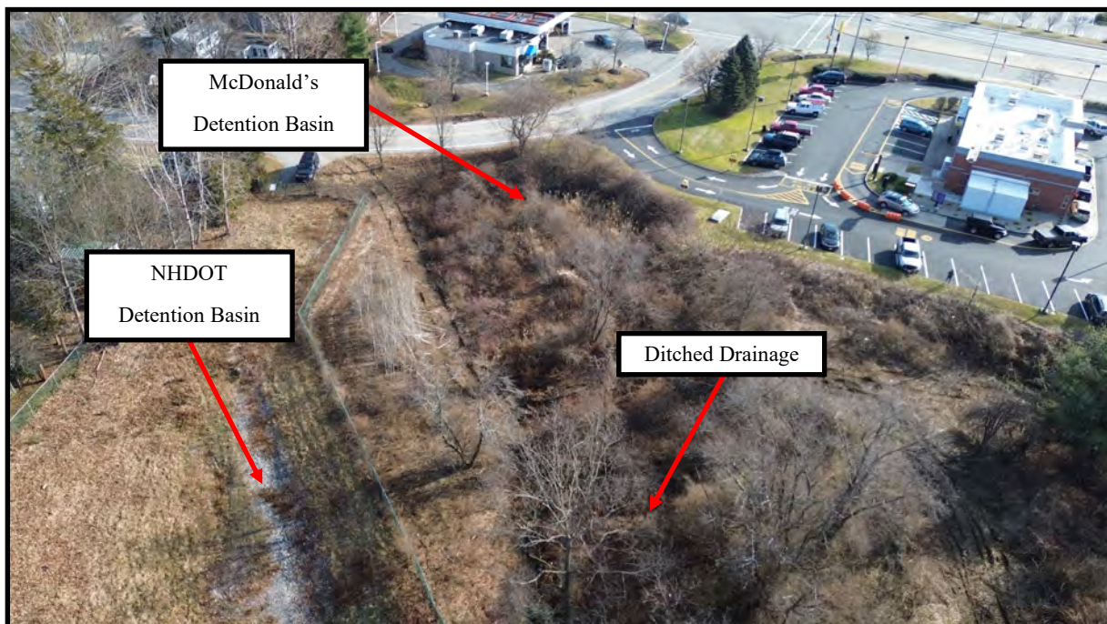
Photo 4: Aerial view of the detention basin located on the abutting NHDOT lot, the abutting McDonald's and its associated detention basin, and ditched drainage located near the northeastern property boundary.
