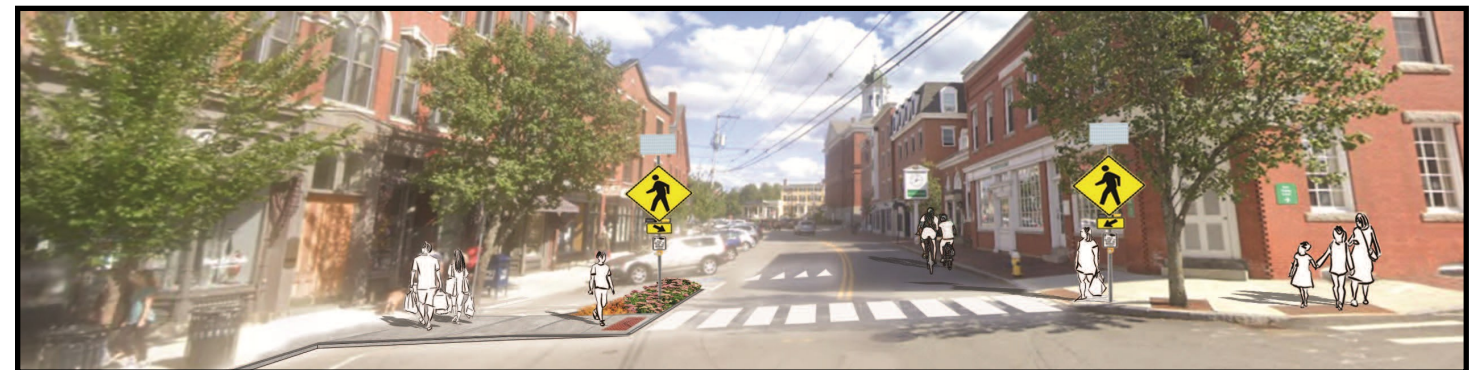
Proposed crossing safety improvement at Water & Center Streets including curb bump-out, signs and flashing beacons. Rendering by LaVerriere Landscape Design
